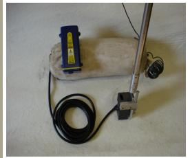
The keyhole tooling utilized to attach anodes and test wires to the gas main include a pneumatic grinder and a furnace/firing controller device that provides placement of the anode wire or test wire in the braze material.
