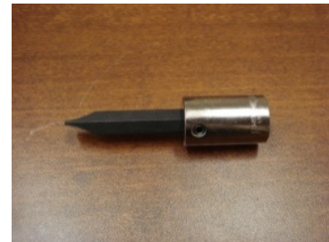
Screw driver bit, #3 x \frac{3}{8} " drive: SRW-3059
