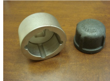
1" Mueller cap installation tool: SRW-3054
