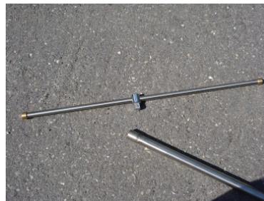
Tee handle ¾" drive w/ 3 ft. handle: GTN-1005
