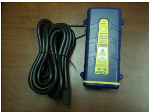
Cadweld control unit w/15 ft. leads: CPS-1416
